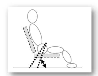
Shell type and aluminium seats with a single crotch belt hole forward of the inside seat back from 11 to 13 inches (279mm to 330mm):
